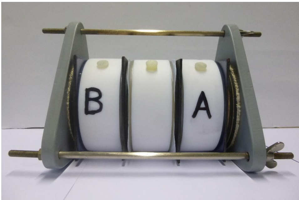
Figure 1: Exemplary setup for migration testing of enamelled test plates (photo: TÜV SÜD Industrie Service GmbH)
